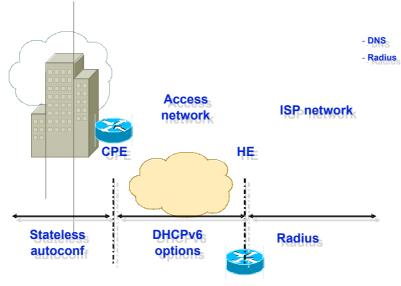
Figure 2-1:Autoconfiguration Overview
