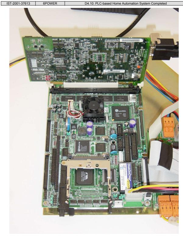
Figure 2-2: PCI PLC Card and Device's Main Board (I)
